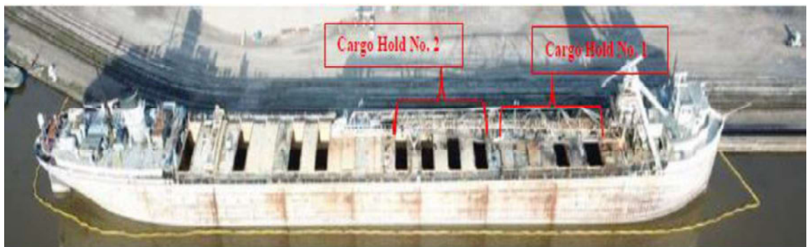
Figure 3. Photograph of Cuyahoga 's hatch covers taken post-fire. Source: Ashtabula Fire Department.
