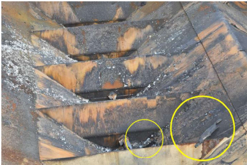
Figure 16. Close up photograph of charred wood scaffolding planks located inside Cuyahoga 's Cargo Hold No. 2. Source: Ashtabula Fire Department.
